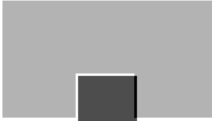
Figure 13.8 Misregistered separations with white gaps
