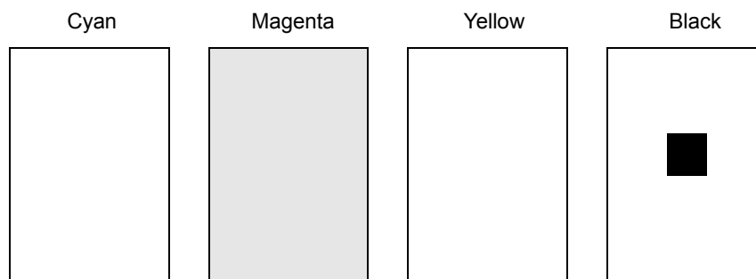
Figure 13.9 Color separations for a simple image, with black overprinting
