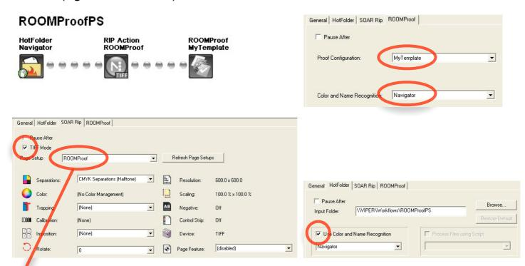
Make a RIP page setup to make CMYK+spot separations at an integer factor of the printer's resolution (to avoid moiré).
