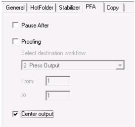
If this control is unchecked, jobs will be left-justified. This Center output control takes precedence over the Center control in the Aspen v2 plugin device dialog.
