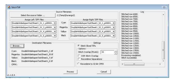
13.3 Press the 'Process' button to stitch the TIFF images together to single recombined TIFF image; carefully inspect result has no misalignment. If instead you do not have the Recombine Separations checkbox, the output will be a stitched TIFF image for each color channel.
