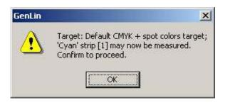
Arrange the target in the direction of the arrow with the first (Cyan) strip under the measuring head and slide the target under the head until it stops. Click OK and feed the target gently through the reader.
