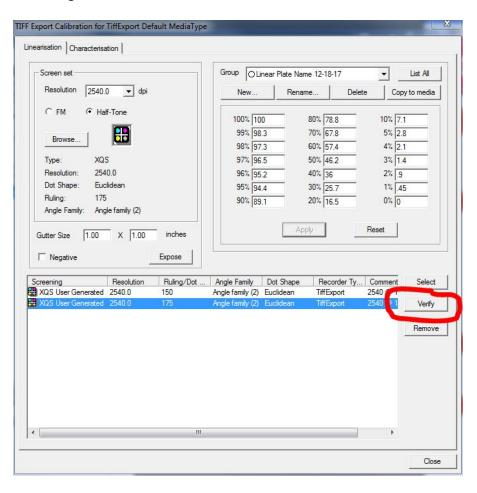
13. The Linear curve is now complete. To apply the curve, select the screens applied to the Linearization Curve from within the job.
