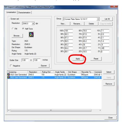
12. You should 'Verify' the new curve by click on the verify button, and run the resulting TIFF through the CTP, and then scan the new chart with the plate reader. If need be, you can then adjust the Linear values to get them closer.
