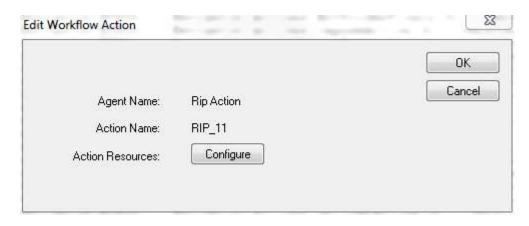
☐ For each, uncheck the 'RIP is local' flag and point the RIP Action at the respective pagebuffer share for the RIP (xpgb1 or xipgb2) and set the instance number in the RIP configuration dialog.
