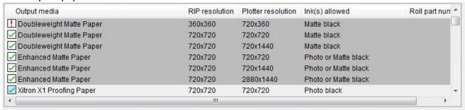
Epson printers all use a starting curve. These listed papers represent those curves. The built-in profiles were made with the appropriate paper selection here.
