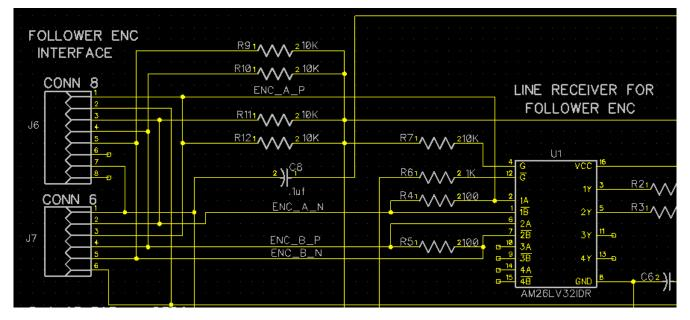
**Belt Encoder 0.1: SIP J7** – This is the input for the rotary optical encoder that monitors the main media belt. Consult the diagram above for connection of the 2 phase (Encoder A and Encoder B) differential input pairs (P & N) that are buffered by U1, a differential line receiver. A similar signal complement is available on J6, the barrel connector version of this interface.
