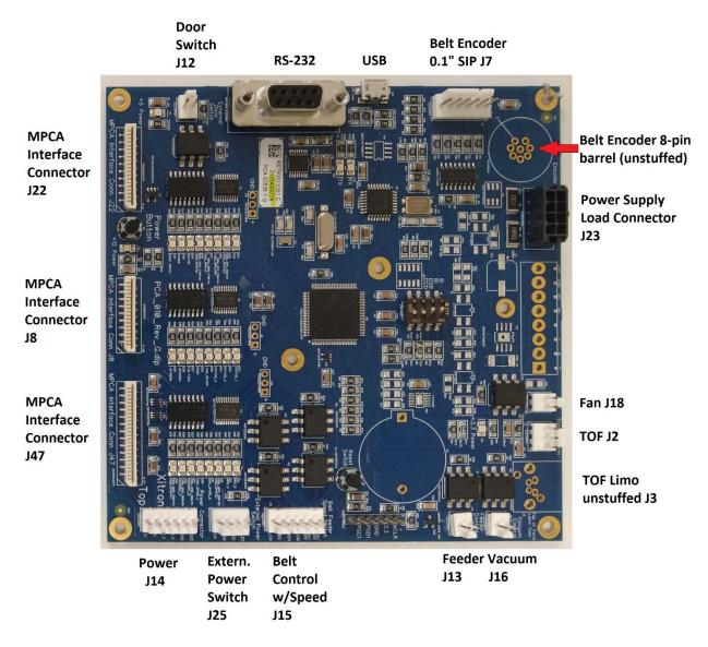
Starting with the connectors that are directly coupled to the HP "Bar in a Box" motherboard:
