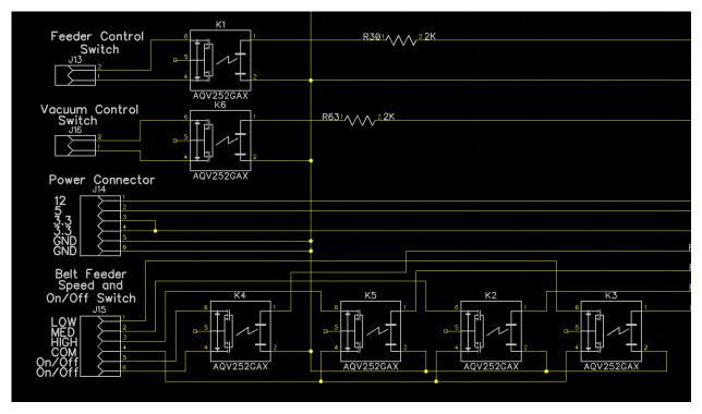
**Feeder Control Switch J13** – This simple "closure" on active can accept up to 60 volts and 2.5 amperes. It is, as with all the AQV252G devices, optically isolated for added protection of the Xitron PCA circuit.
