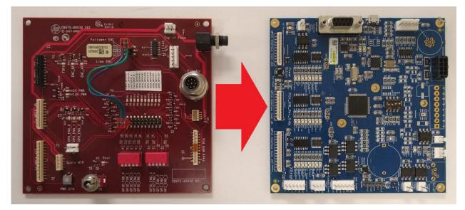
With the addition of a Microchip PIC 24F microcontroller, communications ports, and a plethora of input, output, monitoring, and status signals, the Xitron HP PCA card is a logical choice for OEMs to integrate their own printing solutions around the HP "Bar in a Box" offering.
