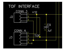
**TOF J2** – This connector is attached to a powered 12 volt sensor that will scan the belt for Top Of Form indications (media present). J2 is implemented as a 0.1" 3-pin Single-In-Line (SIP) connector. Pin 1 is a +12 volt supply line to power the sensor with Pin 3 as the ground. The actual TOF indication (high/low) is returned on Pin2.
