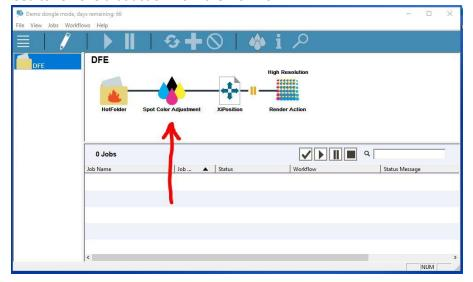
10. To remove the Spot Color Adjustment option, select the edit workflow option.
