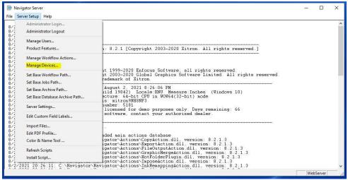
16. Once the Manage devices window opens, there should already be an FI-1000 device created. Select the **"Stop** Thread" button highlighted in the screenshot. This will stop the active threads and allow you to make edits. Edit the device name, IP address of the printer, and the port you are using for the webserver.
