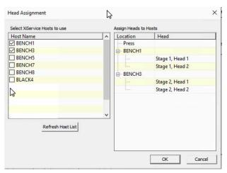
Check the RIP Host PCs to use in the left column. Drag Heads from the Press section to the PC you wish to RIP for that head.
